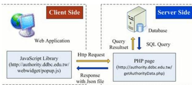
Fig. 5. Communication scheme between client and server through web services.
