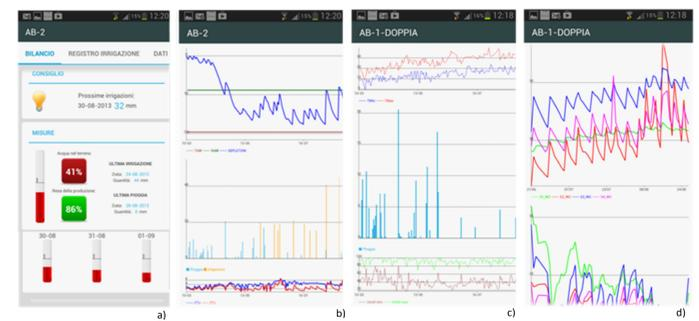
Fig. 4. Example of MOBILE Android application: a) suggestion of the next irrigation (day, amount), with the level of current and projected 3-days changes in soil water content; b) the seasonal trend of soil water depletion, with respect to the RAW threshold, together with the graph of rainfall and irrigations; c) meteorological variables; d) daily trend of soil water content at different depths as recorded by soil moisture sensors.
