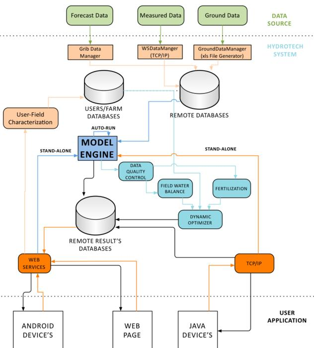
Fig. 3– Data communication and elaboration: general scheme of the HydroTech Information System.
