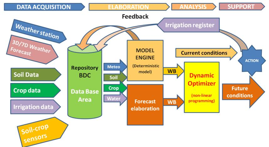
Fig. 1. Data Flow scheme. Multiple data source streams are stored into DB and aggregated in order to obtain the optimal solution for the irrigation/fertirrigation scenario.
